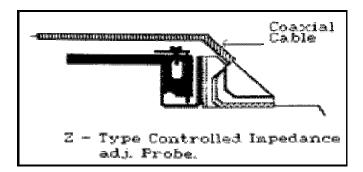
The design illustrated above incorporates all the advantages of the Z adjustable probe combined with an unusual dual impedance front end. These probes are assembled as either 50 ohm or 100 ohm matched impedance paths and offer either single needle or co-planar needles to the DUT. These probes are supplied with a matched impedance coaxial cable especially selected for its small size and flexibility, which is important due to the effect cable stresses and movement may have on probe position.
